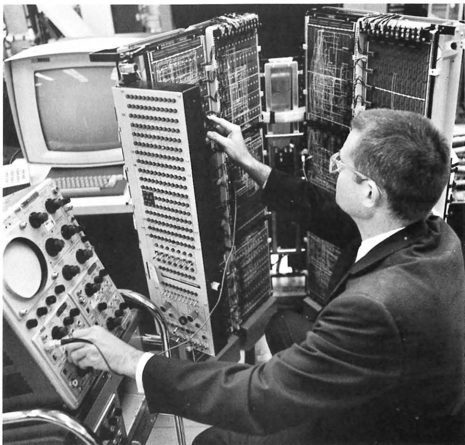
FIGURE 3: The 2250 Model I main control logic is in servicing position. The logic gates swing up and fan out for ease of servicing. A maintenance panel provides trouble-shooting capability off-line from the computer.
