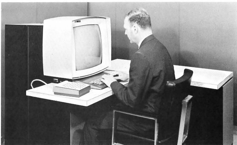
FIGURE 4: The IBM display systems are direct-view CRT display systems designed for single- or multiple-console installations. Multiple units can be separated from their control units by up to 2000 ft. of cable. Detection, tracking and sketching can be performed with a light pen.
