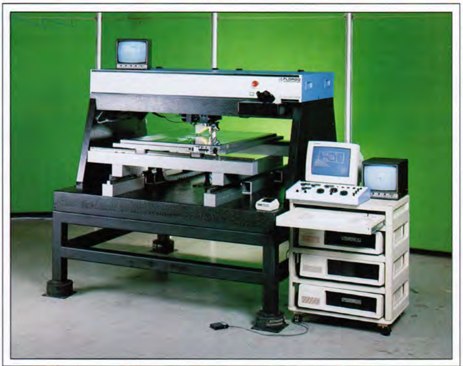
Fig. 3: In FPD substrate processing, bigger is better. Modern laser processing stations can accommodate displays as large as 1 × 1 m.
