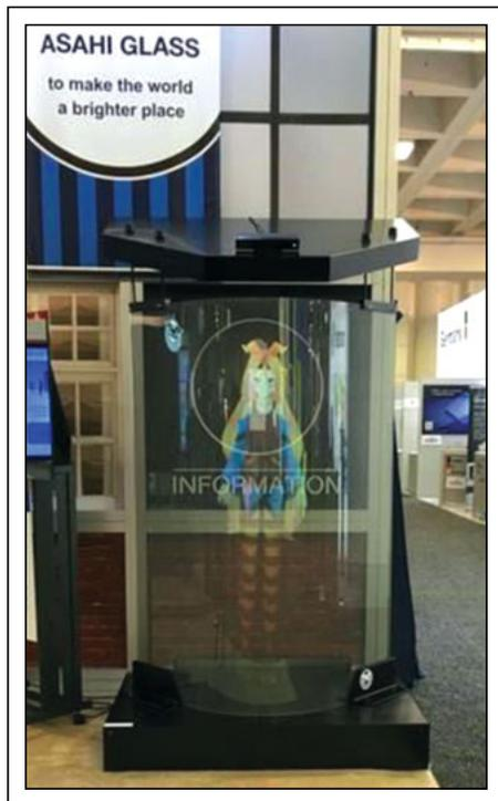
**Fig. 2:** This interactive virtual concierge robot is an example of Asahi Glass Co.'s Glascene technology, in which an image projected onto a transparent glass screen becomes an interactive presentation through motion sensing.
