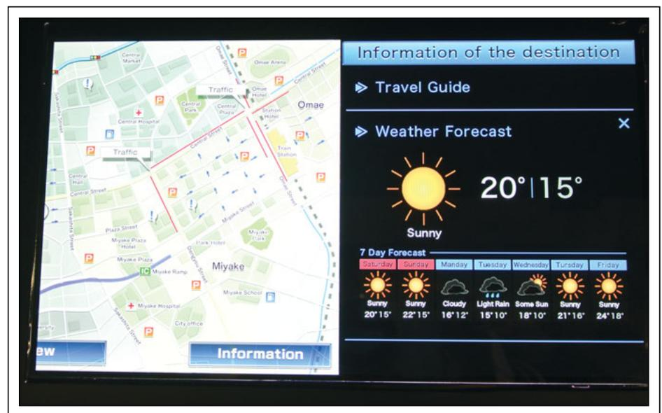
**Fig. 3:** JDI's local-dimmed 10.2-in. tablet display module had a CR of 110,000:1 or above, according to the company. Photo courtesy Jyrki Kimmel.
