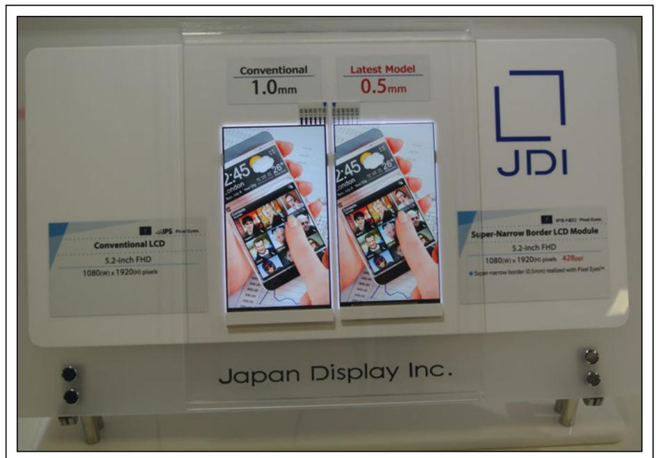
**Fig. 1:** The inactive space at the edges of JDI's super-narrow-border display module (right) is only 0.5 mm wide. The difference from the conventional example (left) is noticeable. Photo courtesy Jyrki Kimmel.
