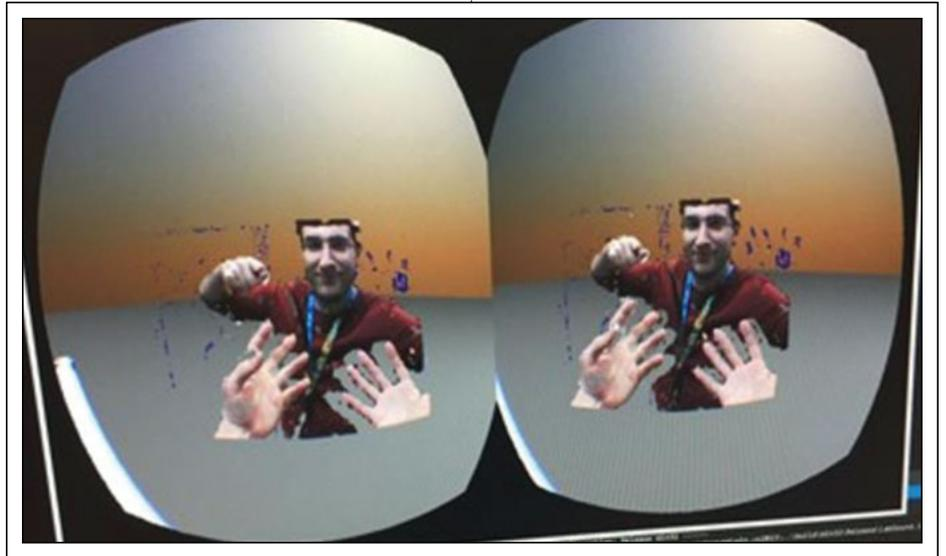
**Fig. 7:** The "merged reality" capability of a device is shown here with integrated Intel RealSense technology.<sup>10</sup> The 3D images of the user's hands as well as a person standing in front of the user are brought into the virtual world. This capability is also used to allow multi-room scale mobility with integrated six-degrees-of-freedom positional tracking to help the user avoid colliding with physical objects.
