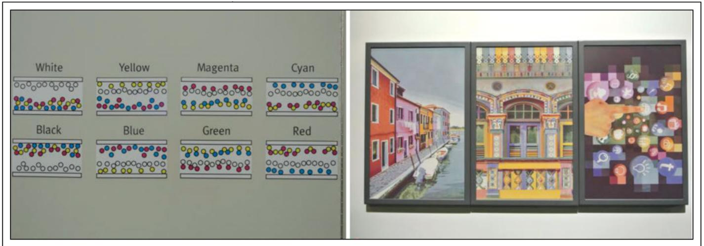
*Fig. 1: E Ink's new color technology uses particles of four different colors within each microcapsule (left) that are controlled in such a way as to create thousands of colors for an unusually vibrant electrophoretic display (right).*
