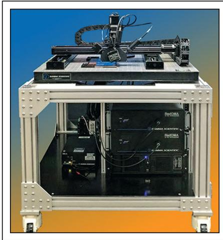
*Fig. 2: Gamma Scientific's Dual Angle Reflectance Measurement System is designed for high-speed automated reflectance measurements of glass for display and architectural uses.*
