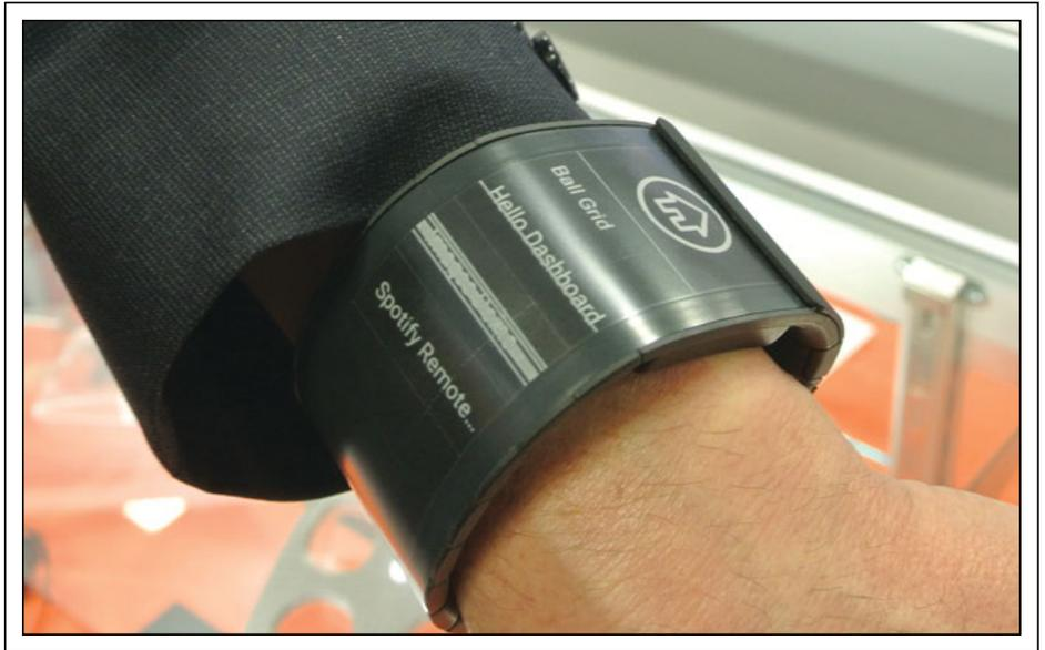
*Fig. 8: The Wove wrist device prototype features an electronic-ink screen integrated with Canatu's carbon-nanobud touch screen. Photo courtesy Jyrki Kimmel.*
