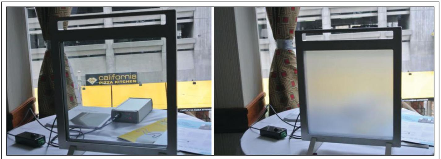
*Fig. 5: Merck demonstrated smart windows that could turn from clear (left) to diffuse (right), courtesy of the company's liquid-crystal-material Licrivision.*
