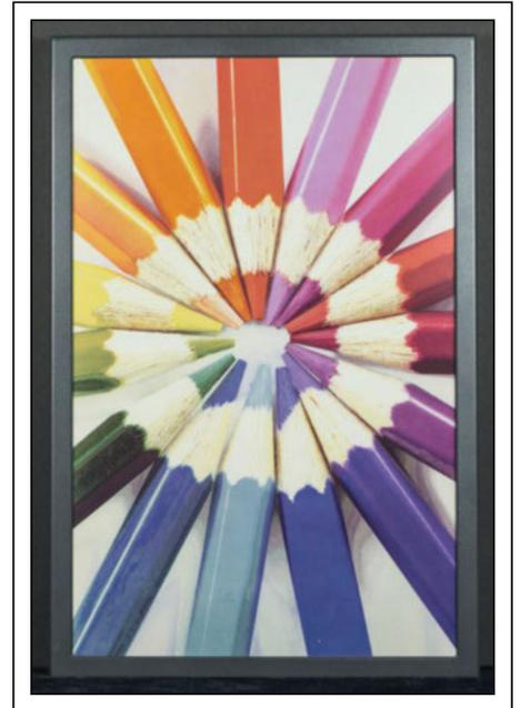
**Fig. 3:** E Ink's new color electrophoretic technology produces color without the use of filters.
