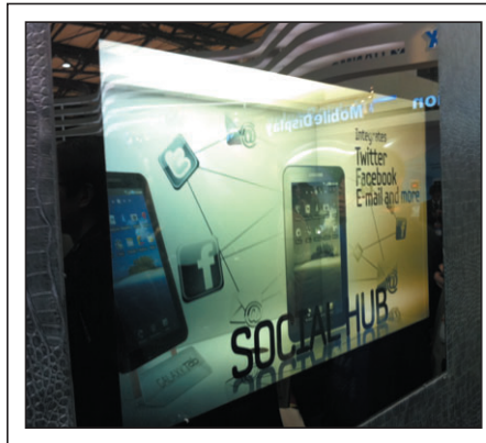
Fig. 1: Samsung's transparent LCD panel will allow retailers to place changing text and graphics in front of physical merchandise, such as these portable display devices.
