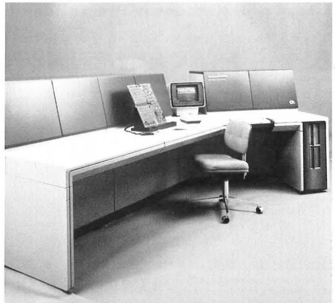
Marathon functional test stations are derived from the Capable 4900 line of real-time functional testers. These stations offer test pattern speeds of up to 16 MHz data rate, 4 MHz test cycle rate, and up to 1024 pins with interchangeable high-speed programmable interfaces.
