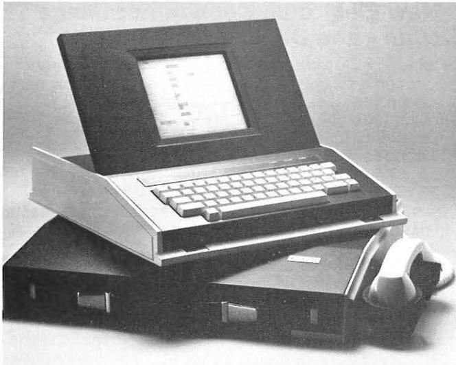
Kylex portable display terminal fits into an attache case because of its compact LCD.
