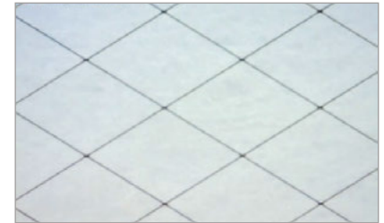
Imbedded Mesh ( \leq 5 OPS, T\% \geq 90\% @ 420-680nm)
