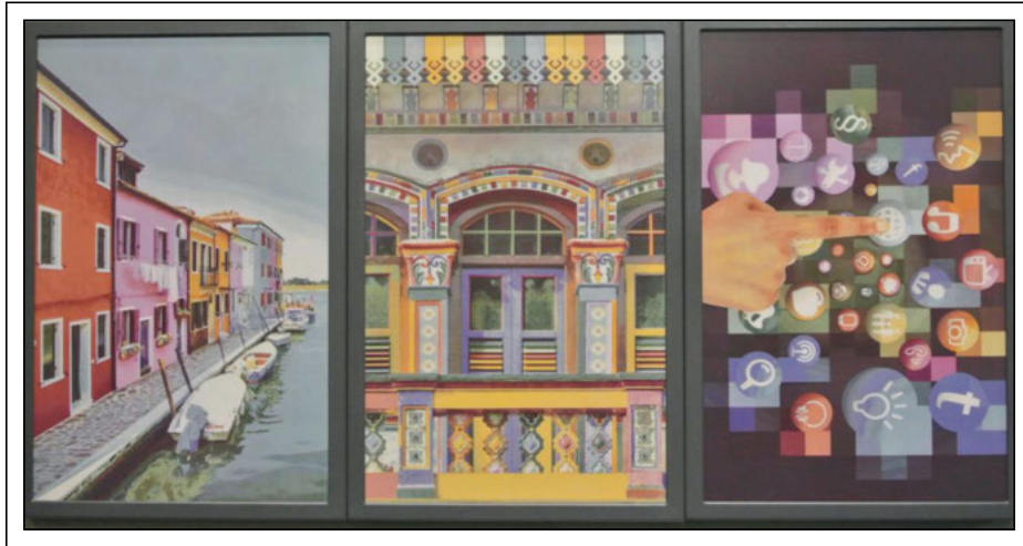
Fig. 3: E Ink's full-color electrophoretic display has four colors of particle and no matrix color filter. (Photo: Ken Werner)
