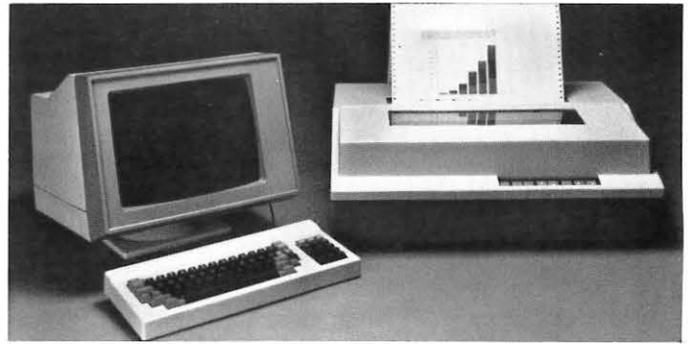
The Envision 230 Advanced Color Graphics terminal incorporates high-level graphics features useful for advanced business and engineering applications. In addition to a full range of scaling, rotating, and area fill features, the model 230 offers a powerful display list capability that allows local storage and manipulation of graphics objects. Objects can be any combination of vectors, arcs, rectangles, circles, polygons and text.
