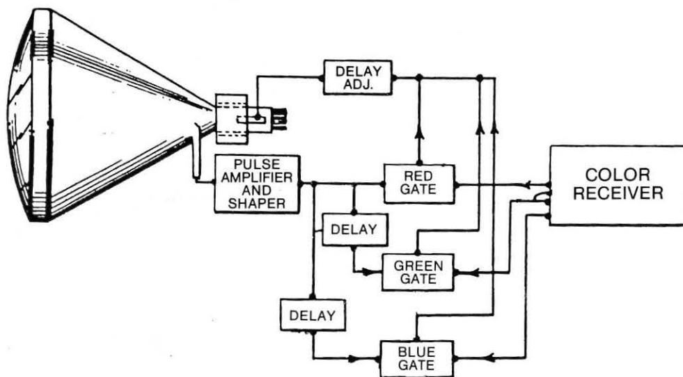
Figure 1. Block Diagram of Beam-Index Color Display System
