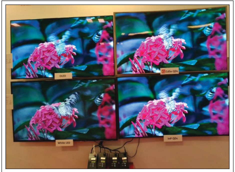
Fig. 1: QD Vision showed side-by-side performance benchmarking of TVs with different technologies demonstrated at the show. Top left: OLED; top right: CdSe QDs (Color IQ); bottom left: white LED; bottom right: InP QDs.
