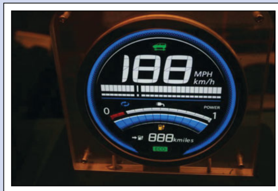
Fig. 1: This Varitronix circular LCD is used in the Nissan Leaf battery electric car. (Photo courtesy Ken Werner)
